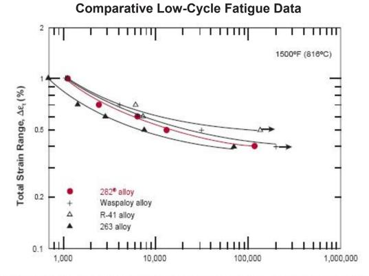
1500°F (816°C), Fully Reversed, R = -1, Waveform = Triangle, Frequency = 0.33Hz, Material: 0.125"(3.2 mm) Sheet\*
