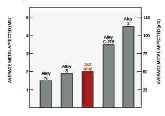
Samples were exposed to a mixture of KCl-KF-NaF salts for a total of 40 hours in service. Temperature was cycled from 1290 to 1650°F (700-900°C) during the course of the exposure.
