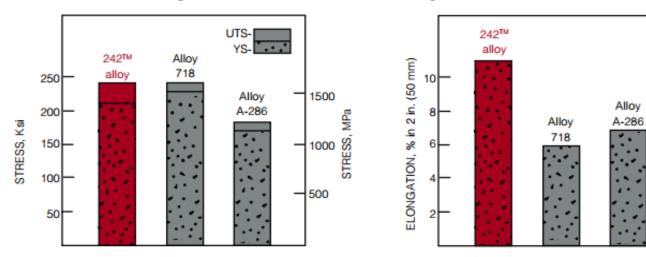
\*Alloys cold-rolled to 40% reduction. 242® alloy aged 1200°F (650°C)/24 hours/AC; alloy 718 aged 1325°F (720°C)/8 hours/FC to 1150°F (620°C)/8 hours/AC; alloy A-286 aged 1200°F (650°C)/16 hours/AC.
