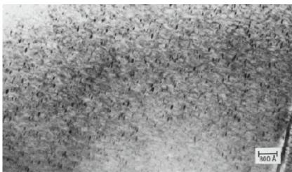
Transmission electron micrograph showing long-range-ordered domains (dark lenticular particles) in 242® alloy. (Courtesy Dr. Vijay Vasudevan, University of Cincinnati). Sample was solution heat treated at 2012°F (1100°C) and aged for 100 hours at 1200°F (650°C).
