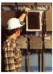
230 retorts operate at 2100°F (1150°C) with a hydrogen atmosphere (inside) and combustion products outside.
