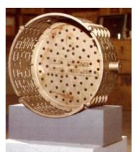
Cast heat-treat basket of 230 alloy in use at Alloy Foundries, Division of the Eastern Company, Naugatuck, Connecticut. Substrate holder and box of 230 alloy resist temperatures of 1650°F (900°C) during the production of semiconductors.
