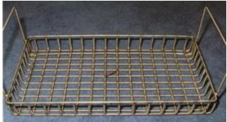
Fabricated heat-treating basket for vacuum furnace application to 2300°F (1260°C). Made from 1/2-inch (12.7 mm) diameter 230<sup>®</sup> bar.
