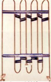
Resistance-heated 230<sup>®</sup> superheater tubes at the Penn State Applied Research Laboratory. Used to produce about 1625°F (885°C) high-pressure steam.
