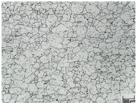
Etchant 95ml HCl plus 5 gm oxalic acid, 4 volts
