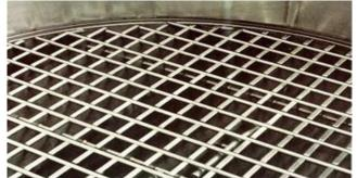
Nitric acid catalyst grids support made from HAYNES<sup>®</sup> 230<sup>®</sup> alloy plate and bar. Excellent creep strength at 1700°F (927°C) makes the alloy highly suitable for this application.
