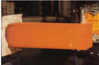
This horizontal electrically fired 230<sup>®</sup> retort replaced an alloy 600 retort which lasted only an average of eight months in 1400 to 2200°F (760 to 1205°C) service in hydrogen atmosphere. The 230 retort was still in excellent condition after 24 months service, as shown.
