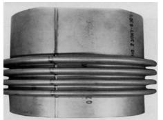
Prototype 230<sup>®</sup> high-temperature expansion bellows made of 0.020-inch (0.5mm) thick sheet in a catalytic cracker configuration.
