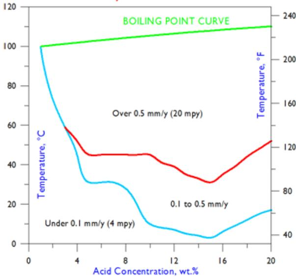
Iso-Corrosion Diagram for G-30 Alloy in Sulfuric Acid
