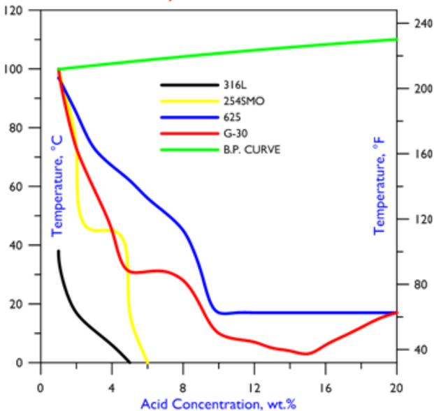
Comparison of 0.1 mm/y Lines in Sulfuric Acid
