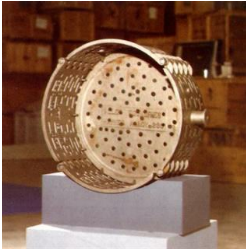
Cast heat-treat basket of 230 ® alloy in use at Alloy Foundries, Division of the Eastern Company, Naugatuck, Connecticut.
