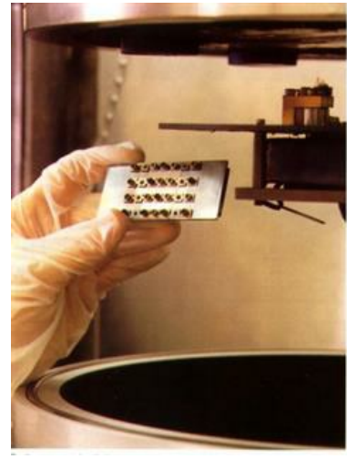
Substrate holder and box of 230 ® alloy resist temperatures of 1650°F (900°C) during the production of semiconductors.
