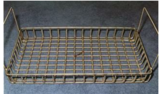
Fabricated heat-treating basket for vacuum furnace application to 2300°F (1260°C). Made from 1/2-inch (12.7 mm) diameter 230 ® bar.
