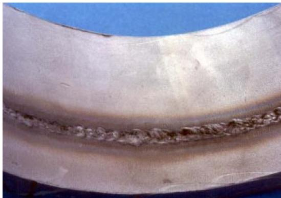
Lack of proper shielding produces a condition which is often referred to as "sugar" of the root pass. An example of such a root-pass weld, made on an 8" diameter HASTELLOY<sup>®</sup> C-22<sup>®</sup> alloy pipe, is shown in Figure 1. An unacceptable root pass is characterized by a black, crusty appearance of the weld metal on the inside (root) of the pipe and an irregular root cross-section.
