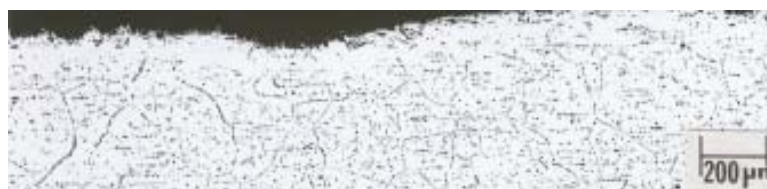
Type 304 Stainless Steel Average Metal Affected = 8.1 mils (205 µm)
