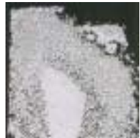
HASTELLOY X alloy Average Metal Affected = >22 Mils (560 µm)/Side
