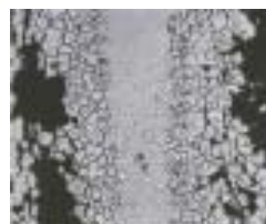
Alloy 800H Average Metal Affected = 23.2 Mils (590 µm)/Side
