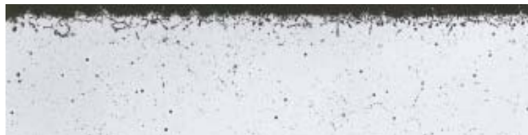
RA330 alloy Average Metal Affected = 4.3 mils (110 µm)
