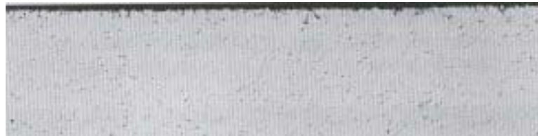
HAYNES 556 alloy Average Metal Affected = 1.1 mils (20 µm)
