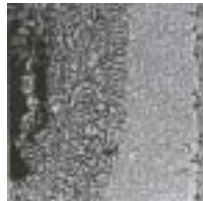
INCONEL alloy 601 Average Metal Affected = >22 Mils (560 µm)/Side
