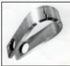
HASTELLOY B-2 alloy Annealed + 1 hr at 700°C (Intergranular cracking, 3 hours)
