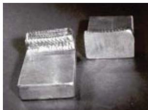
ULTIMET® Weld Overlay Six-Layer Deposit, Crack-Free
