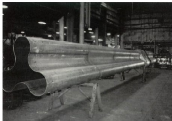
Large Welded retort fabricated from 0.375 inch (9.5 mm) HR-160 ® plate
