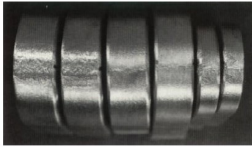
Typical face, root and side bends for HR-160 alloy. The plate thickness was 0.5 inch (12.7 mm) and the bend radius 1.0 inch (25 mm) (2T radius)
