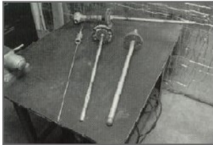
Many waste incineration and chemical process facilities have used HR-160 ® thermocouple protection tubes with outstanding success. Life extensions greater than 10X compared to Ni-Cr alloys and stainless steels are common.
