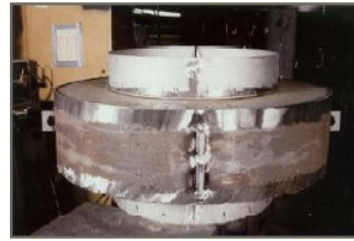
Lining (inner cylinder) of exhaust ducting in pulp and paper recovery boiler made from HR-160 ® alloy. Outer shell is carbon steel.
