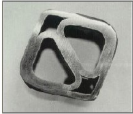
Cross-section of HR-160 ® flue-gas stack Rosemount Annubar ™ averaging pitot tube for waste incineration and chemical process industries.
