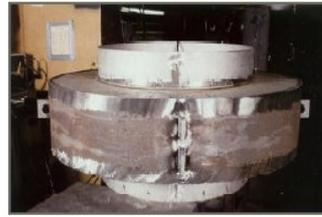
Lining (inner cylinder) of exhaust ducting in pulp and paper recovery boiler made from HR-160<sup>®</sup> alloy. Outer shell is carbon steel.
