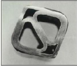
Cross-section of HR-160<sup>®</sup> flue-gas stack Rosemount Annubar<sup>™</sup> averaging pitot tube for waste incineration and chemical process industries.
