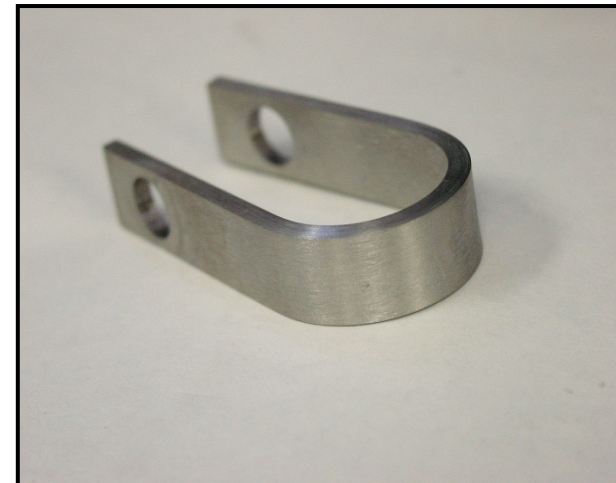
HYBRID-BC1 Alloy (No cracking after 1008 h)
